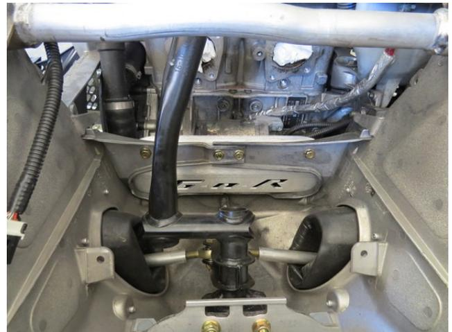
11. Install the two M6x20 bolts and nuts in these holes and torque to 106 (in-lbs).
