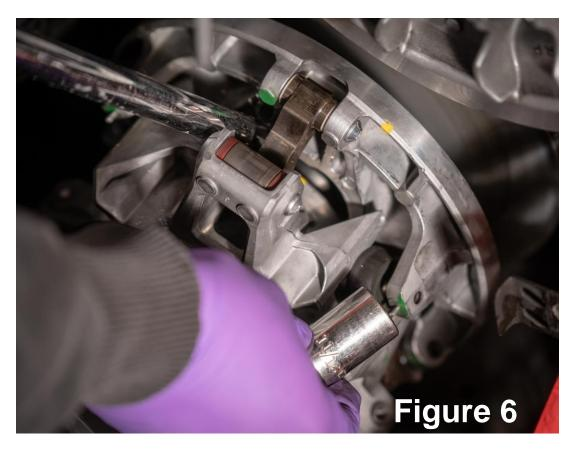
**8.** Reinstall the clutch belt and check deflection. Addition or removal of weight magnets for fine tuning of clutch operation can be performed by opening the clutch using the same technique described in these instructions.
