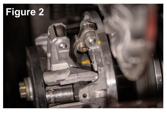
4. The clutch is now open far enough to access the clutch weights. Remove the factory clutch weight/clicker assembly by loosening the pin retaining screw with a T-25 Torx bit until a small gap equivalent to approximately 3/8" of threads showing and GENTLY drive the tapered pin from the clutch as shown in figure 3
