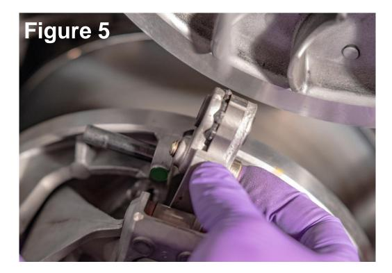
Rotate the clutch and repeat steps 4-6 until all 3 weights have been swapped, then using the 1/2" extension pry the clutch open and remove the 11/16" socket as per figure 6. (Avoid opening the clutch too far to prevent binding of the weights on the clutch rollers)
