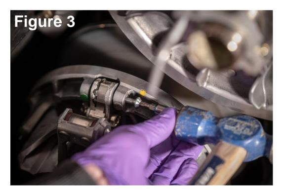
5. Once the tapered clutch pin is loose from the clutch body completely remove the retaining screw and drive the pin far enough to free the weight or the pin can be fully removed if desired. The factory weight will now slide free from the clutch body as seen in **figure 4**
